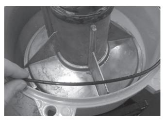
**Step 2** – Remove the casing O-ring.
