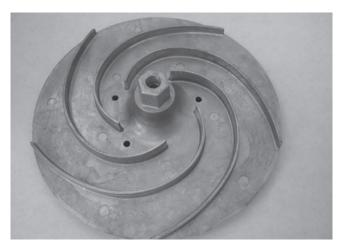
Step 4 – Screw on the back half of the impeller, the impeller has a hex on the shaft that takes a spanner or socket (17mm) to tighten it down.
