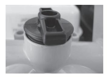
Step 10 – Fit the drain plug and priming plug, use a small amount of water based lubricant for a more secure fit. If a pressure gauge needs to be fitted drill a small hole in the centre of the priming plug & screw the gauge in. The hole should be 1/4 inch in size.
