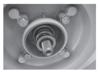
Step 3 – Fit the mechanical seal and push it all the way down to mate with the stationary seal face. This can be made easier by removing the grommet from the mechanical seal, slide the seal onto the shaft & then place the grommet back in position on the mechanical seal.
