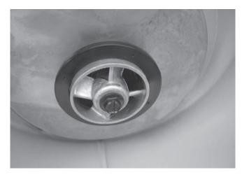
**Step 5** – Fit the front half of the impeller over the rear section and tighten it down with a self tapping bolt using a socket (13mm), the torque setting is 14-16nm then fit the impeller neck ring.
