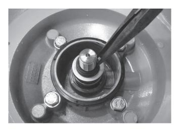
Step 6 – To remove the mechanical seal lift it off the shaft. If the mechanical seal is too tight to remove by hand use a pair of pointy nose pliers to remove the grommet in the middle of the seal, this will then allow the rest of the seal to be lifted up. Check the seal face for wear or abrasives.
