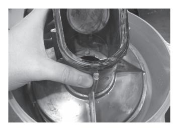
**Step 3** – Remove the diffuser complete with flap valve; this can be lifted out by hand.
