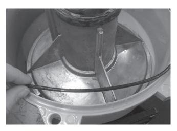
**Step 7** – Fit casing O-ring in place.
