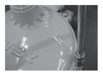
**Step 8** – When fitting the front casing the pins on the inside should sit around the gasket holding it in place. Fit the bolt with the flat washer under the head and tighten the assembly in a criss cross pattern with a socket (14mm or 9/16 AF), torque setting is 22nm.
