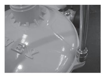
Step 1 – Remove the front casing bolts using a socket (14mm). Do not remove the bolts individually, instead loosen all the bolts before removing any as this keeps the compression on the casing even.
