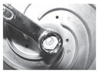
Step 5 – With the screwdriver still locking the cup coil of the motor in place use a ring spanner (17mm) to remove the back of the impeller. If necessary hit the spanner a sharp tap with a soft head mallet to loosen the impeller similar to the procedure with the impeller nut.
