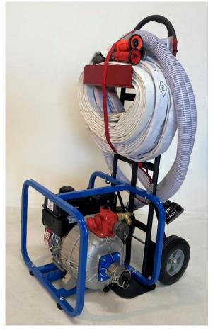
Fire Pump frame is carried on 2-wheel equipment cart and can be removed from cart for transport by SUV or truck.
