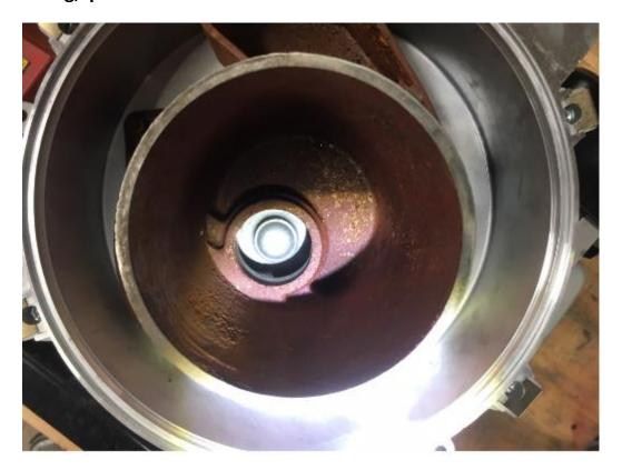
A2) Using a socket wrench, the impeller can be rotated. Socket should be 1". Insert the socket using an extension, and push the socket onto the rounded fitting. Moderate pressure may be necessary to push the socket onto the cap so the socket "grips" the cap. Below is diagram of how the socket is positioned on the impeller.
