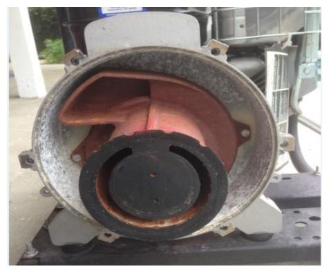
non-petroleum cleaner to remove calcium deposits that may interfere with seal.
