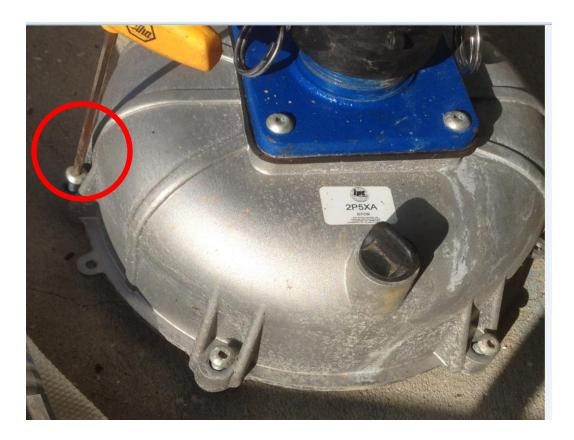
9) If the stainless steel retainers holding the nuts on the pump case come loose, press them back over the nuts. If the retainer comes off, expand them slight when pressing them back over the nut.
