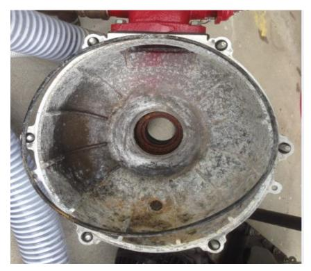
Take care to not stretch the O ring when cleaning it – if it stretches, it may not seal properly when replaced.
