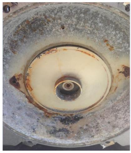
B6) Impeller is removed by rotating counter-clockwise, with the engine shaft not rotating. This is not easy – requires penetrating oil, a gear puller, and patience. Recommend you get assistance from a Briggs repair shop to remove it, if necessary.
