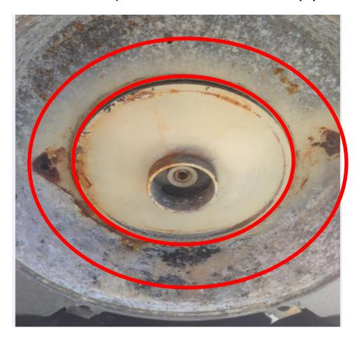
B8) Sand/polish the outside surface of the impeller's hub to remove any corrosion.
